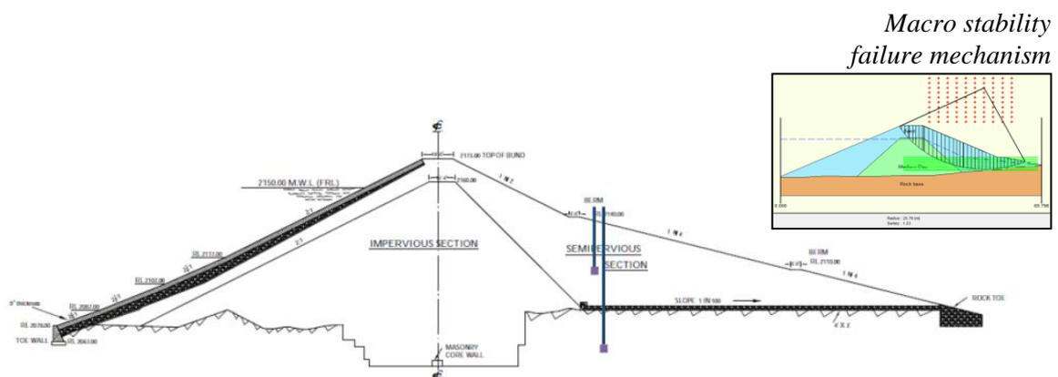
**Figure 9. Instrumentation of Saddle dam 1 with a pore-water pressure sensor in the dam body and in the dam foundation, including considered failure mechanism**
