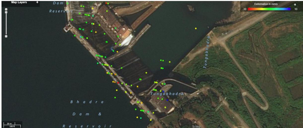
**Figure 5. Main dam deformation (period 29 September 2016 to 11 March 2018)**
