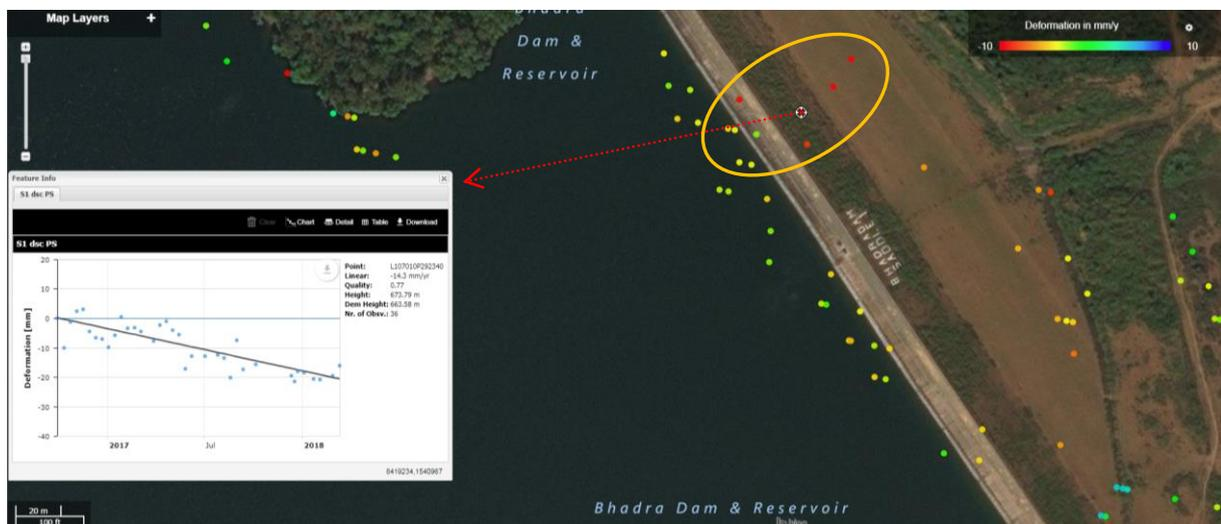
**Figure 6. Saddle dam 1 deformation (period 29 September 2016 to 11 March 2018)**
